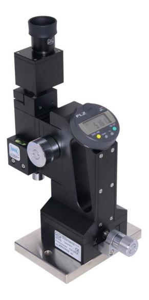
The FLZ alignment tester is a transportable microscope for the alignment of machine guides.
